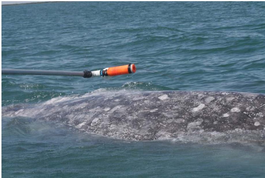
Figure 4. Bio-probe tag with floatation unit (orange) and suction cups (white circles) at the end of the deployment pole
