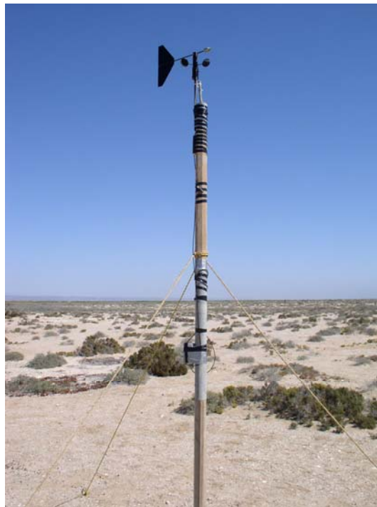
Figure 7. HOBO wind station sampling direction and speed at Punta Piedra
