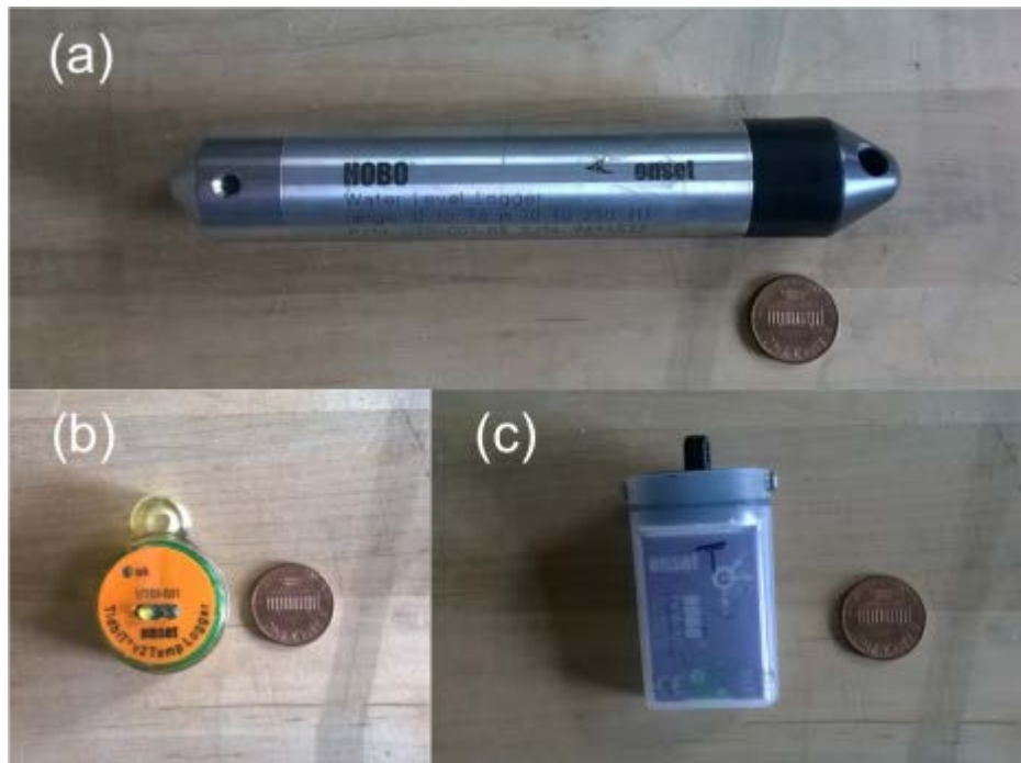
Figure 3 – HOBOWare data loggers (a) Water level logger (b) Tidbit temperature logger (c) Inclinator.
