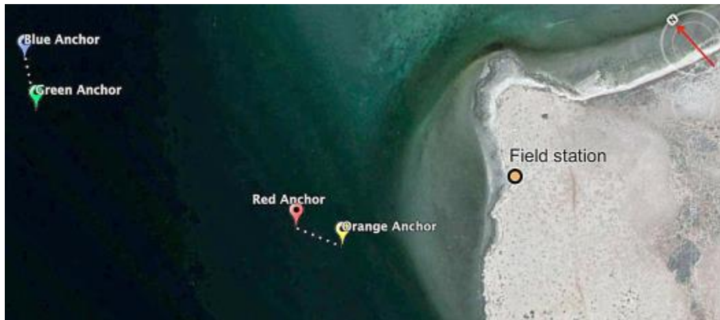
Figure 10. The orientation of hydrophone arrays to localize the source of whale calls in front of the observation tower on Punta Piedra in Laguna San Ignacio.
